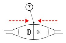
7 Attach the Smart Wrap™ to the Umbilical of the Kelvi Pro™ Series Console. An audible click will be heard when the connectors engage. Use Air Control buttons to adjust fit. To disconnect, press the Release button and pull the connectors apart.
